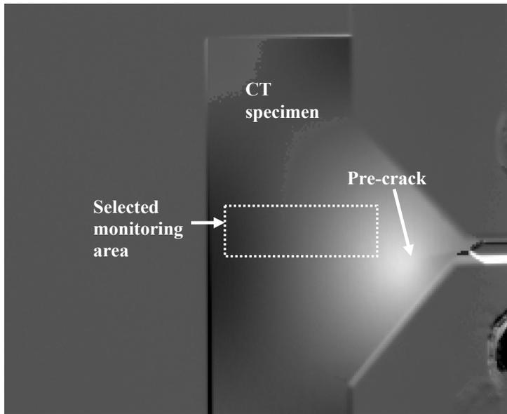
**Fig.5a** CT specimen showing the selected area for thermographic monitoring.
